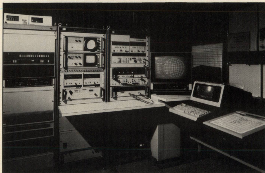
Fig. 1 PLANA/1000 hardware configuration using HP-8409B with HP-1000 computer system and color graphics subsystem.
